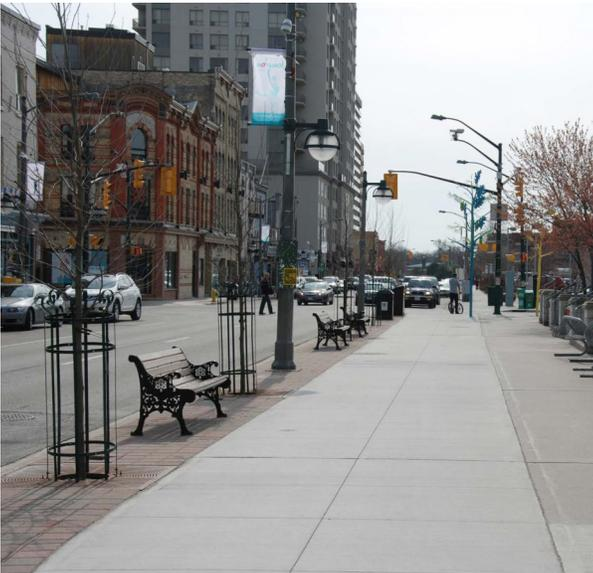
A variety of **pedestrian amenities** including seating, pedestrian-scale lighting, waste receptacles, and trees positioned adjacent to the pedestrian clearway in London.
